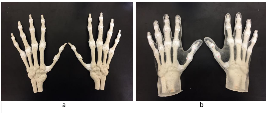
Figure 32: (a) The final design of the finished bone structure (3 rd generation). (b) The casted right and left Gel #4.3 surrogate hands.
