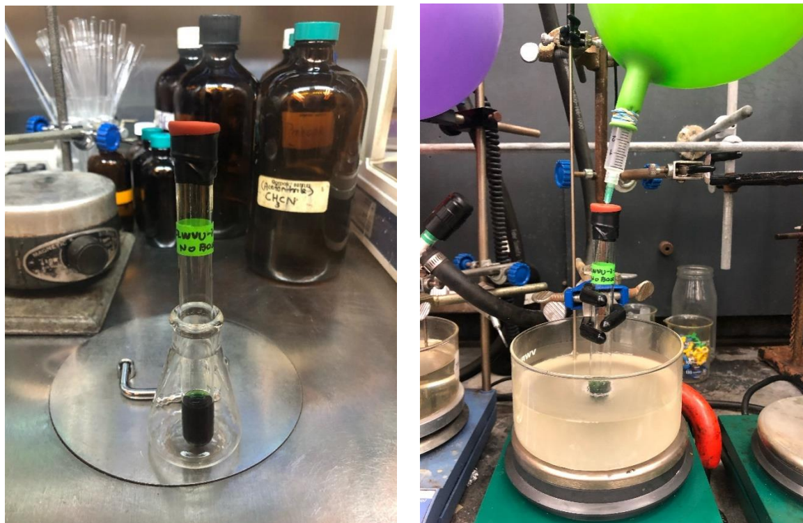
Figure 3.2. Reaction set up for parameter assessment studies. (a) Preparation of the reaction mixture inside the glovebox. (b) Final reaction setup inside a fume hood with an air balloon.
