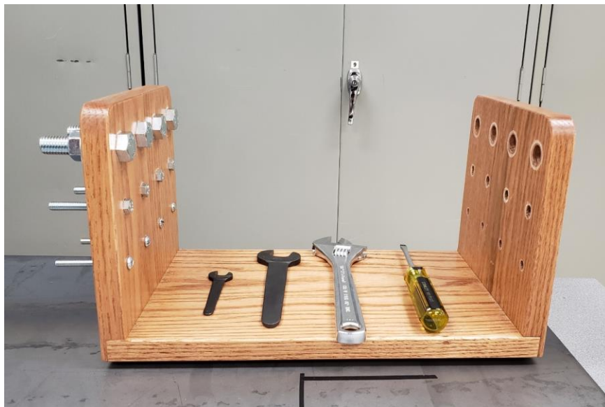
Figure 10: Hand Tool Dexterity Test Apparatus
