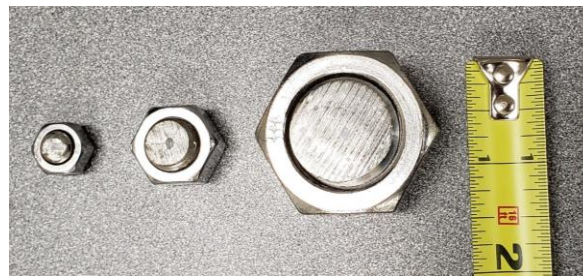
Figure 5: Hexagonal Bolts used as Targets in Test-1
