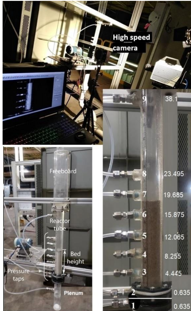
Figure 8. Cold flow experimental setup
