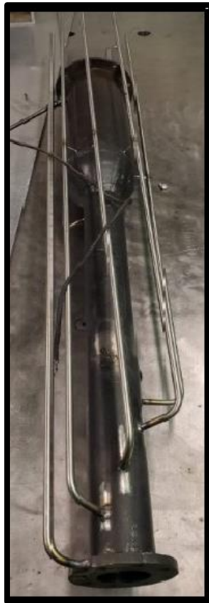
Figure 13. BFBG reactor. The smaller diameter tubes were used to measure the pressure at various bed heights.
