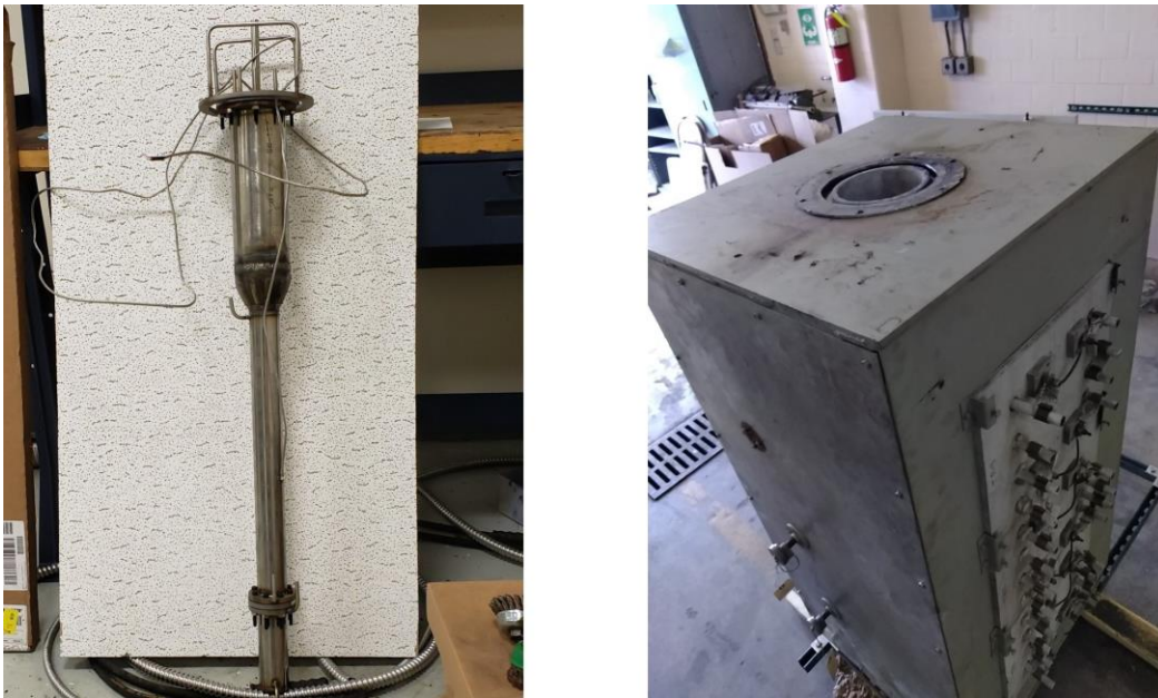
Figure 14. Bubbling fluidized-bed reactor (left) and high-temperature furnace (right)
