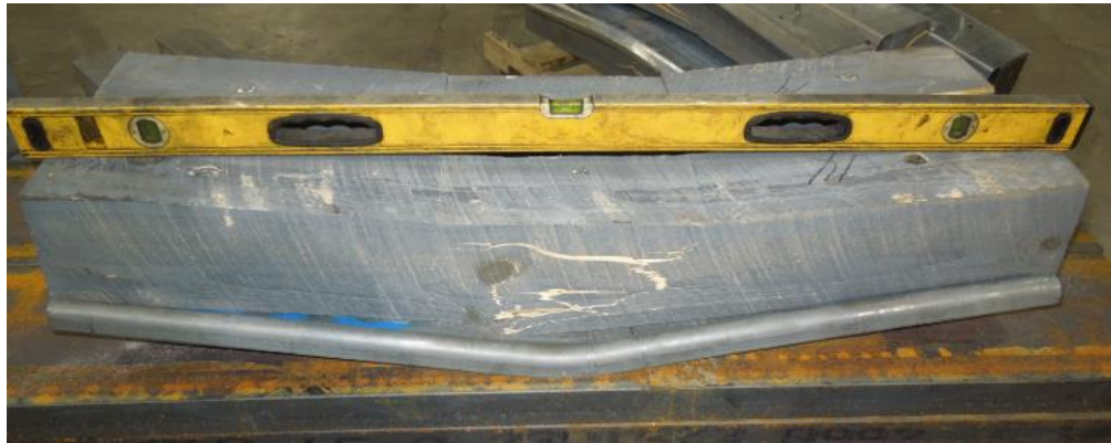
Figure 2.7 - Deformed specimen after impact.
