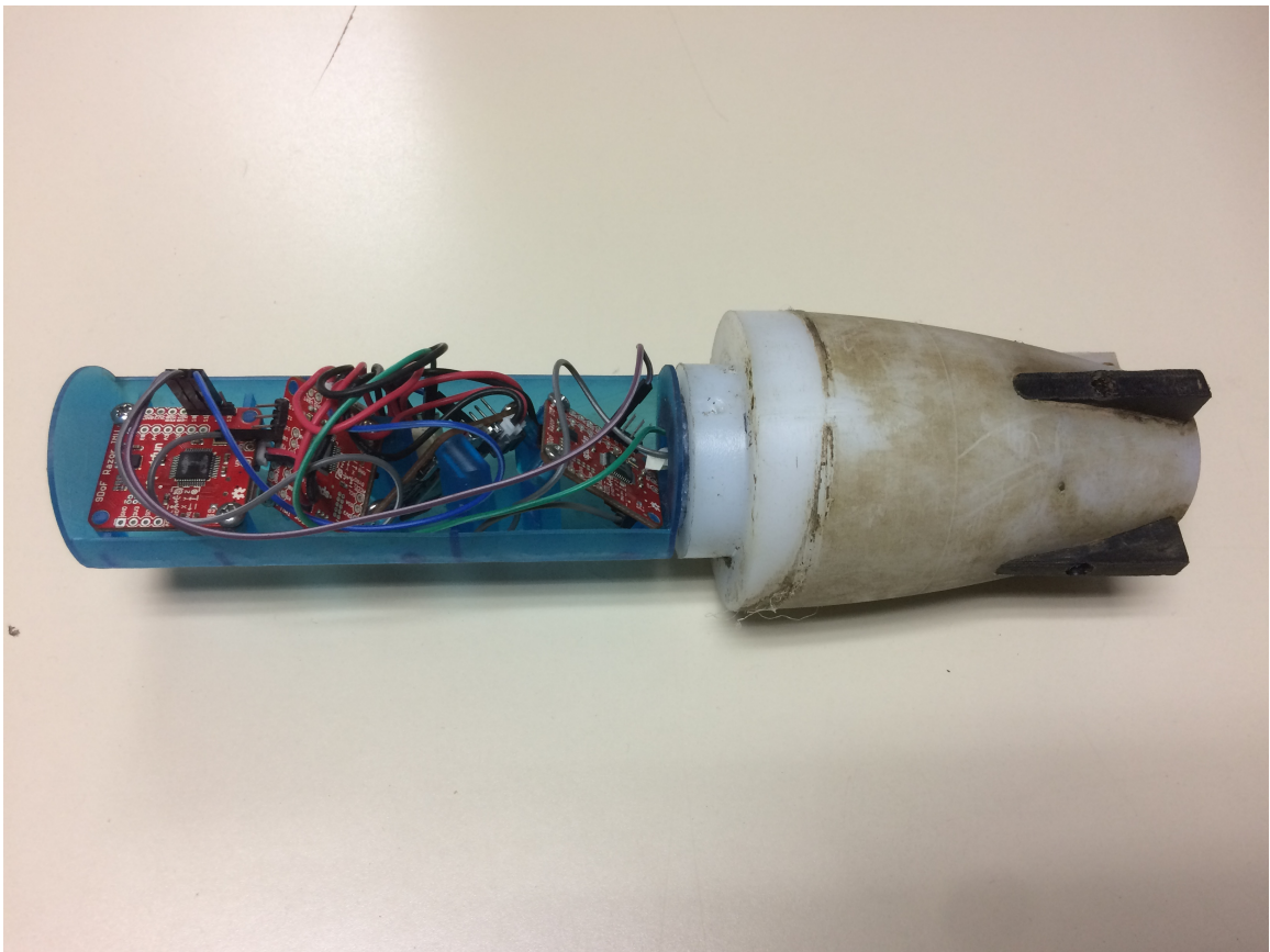
Figure 2.9: Instrumentation payload with IMUs wired together and placed in the tail cone of the flight vehicle
