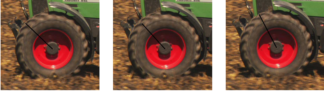
(a) Current picture (POC N), (b) reference picture 0 (POC N-1), wheel angle 136 (c) reference picture 1 (POC N-4), wheel angle 118
