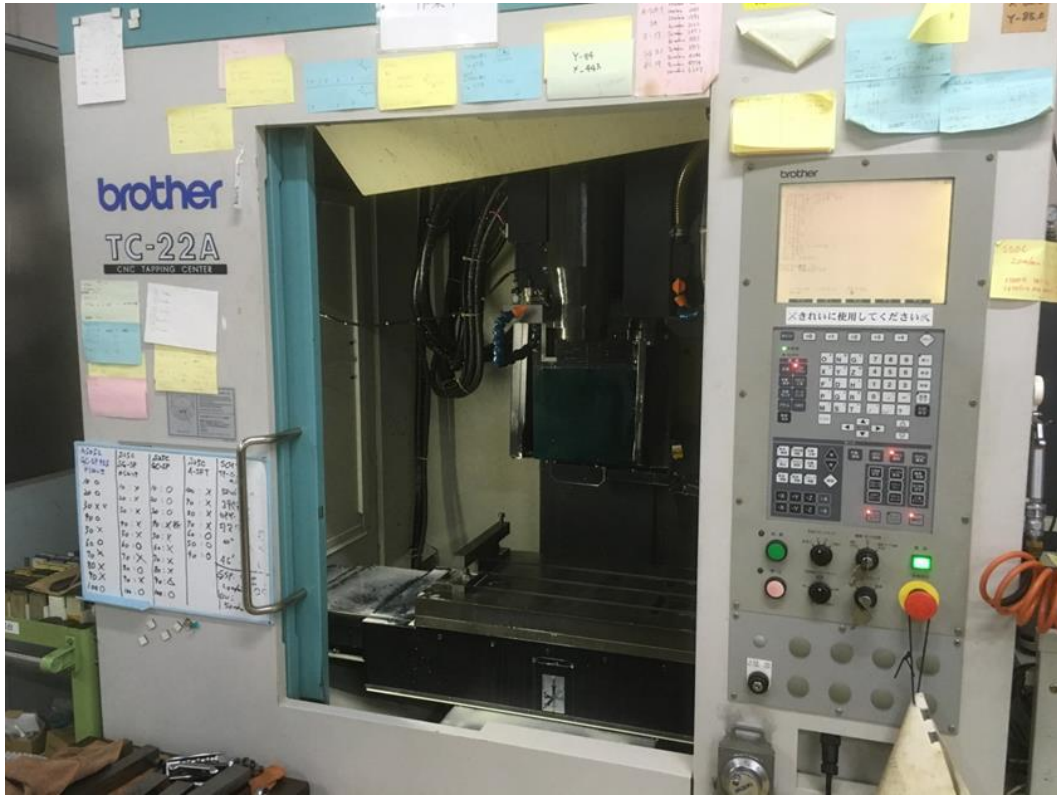
Fig. 2-4 CNC tapping center used for constant feed rate drilling
