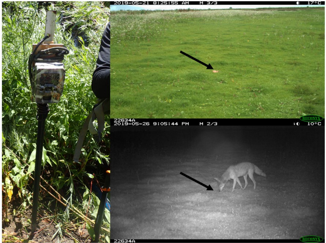
Recoynx PC900 set-up at Central Valley sites. Cameras were attached to the top (~1 m) of a T-post and stabilized using a board, bungee cords, and cable locks (left). T-posts were angled down to have cameras face the ground where bait was placed. A can of fishy cat food was emptied in the middle of the camera frame and spread around over covered with vegetation to prolong animals near camera sites. Black arrow points to bait location during camera set-up (top-right) and during a coyote detection 5 days later (bottom right).
