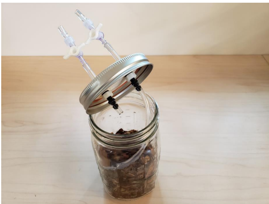
Figure B1. Picture of open incubation chamber with woodchips
