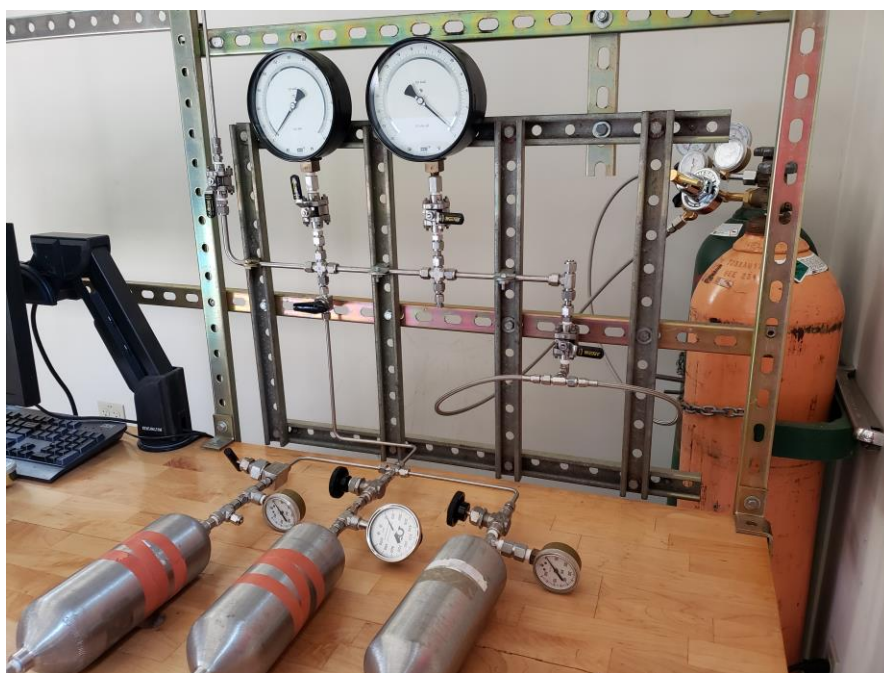
Figure B2. Picture of gas mixing manifold
