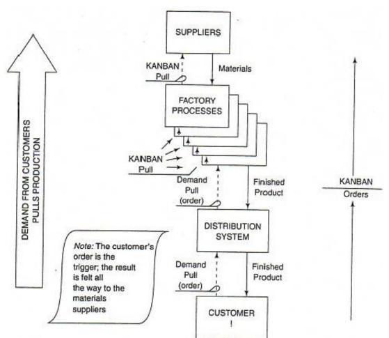
Figure 2: Pure pull or JIT system [3]
