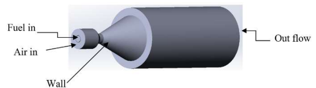
Figure 5. Schematic for specifying boundary conditions
