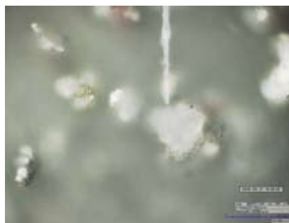
Fig. 15. Tubular molecule aggregates in fullereniferous carbon-black (11 wt. % C 60 ) after cavitation 15000 rpm. Microscope magnification a) 2800 x , b) 1400 x
