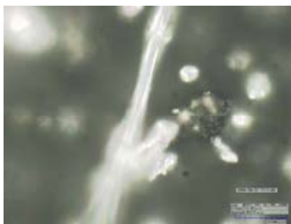
Fig. 15. Tubular molecule aggregates in fullereniferous carbon-black (11 wt. % C 60 ) after cavitation 15000 rpm. Microscope magnification a) 2800 x , b) 1400 x
