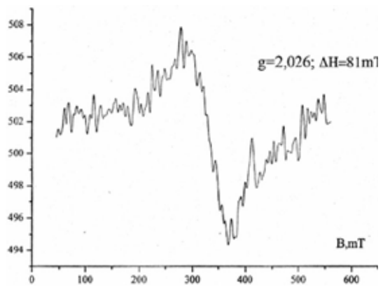
Fig. 20. The EPR spectrum of diamond-bearing carbon-black after cavitation processing
