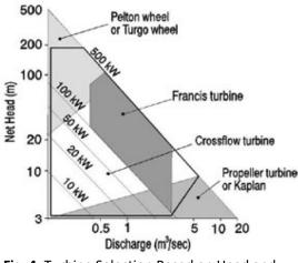
Fig. 4. Turbine Selection Based on Head and Flow Rate [16]
