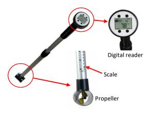
**Fig. 2.** Flow velocity probe for flow velocity measurement
