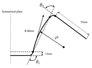
Fig. 8. Springback angle measurement [42].
