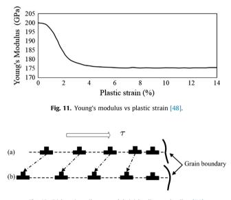
Fig. 12. Dislocation pile-up model; (a) loading; unloading [50].
