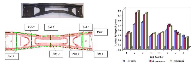
Various experimental techniques and procedures have been developed to analyse and review springback in sheet metal. Among
