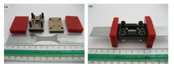
Fig. 10. Experimental apparatus for tension-compression test; (a) dismantled; (b) assembled [47].
