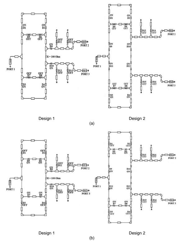
Figure 4. (a) Circuit configuration of power divider at 2.5 GHz and (b) circuit configuration of power divider at 3.5 GHz
