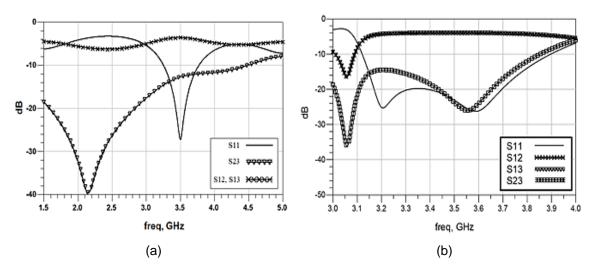
Figure 7. S11, S12, S13, S21, S31 and S23 results for modified WPD (a) design A and (b) design B at 3.5 GHz.
