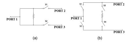
Figure 1. The circuit configurations of power divider with SPDT switch function in (a) design A and (b) design B.
