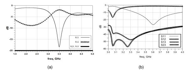
Figure 9. Simulation result, S11, S12, S13, S21, S31 and S23 for SPDT switch (a) design A and (b) design B at 2.5 GHz.
