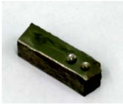
Fig. 1. The Illustration of Hadfield manganese steel sample that have been subjected to dynamic stressing 3000 kg on adjustment of hardness test by Brinell
