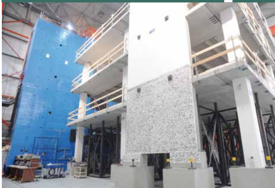
The European Laboratory for Structural Assessment (ELSA) is capable of testing the behaviour of buildings of up to five storeys high when exposed to earthquakes.
