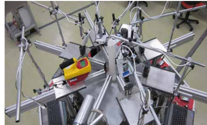
Reference instruments used to record data in parallel to instruments under testing as part of ITRAP+10.
