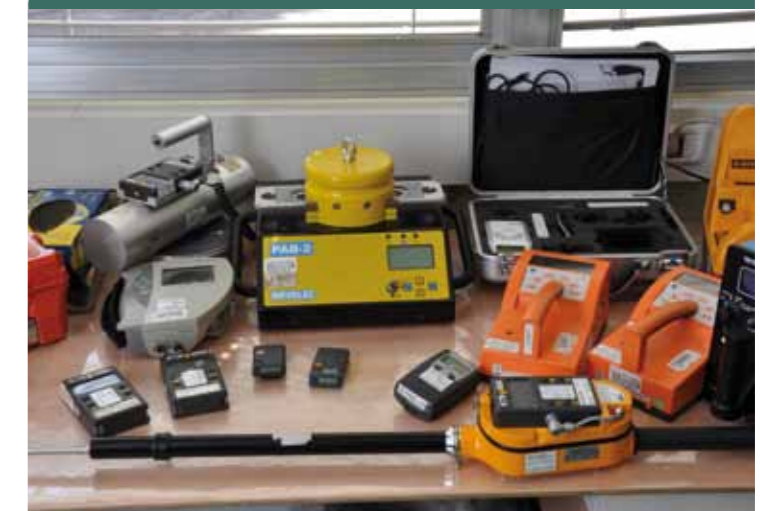
The Illicit Trafficking Radiological Assessment Program +10 (ITRAP+10), inaugurated by the JRC, tests commercially-available radiation detection equipment.
