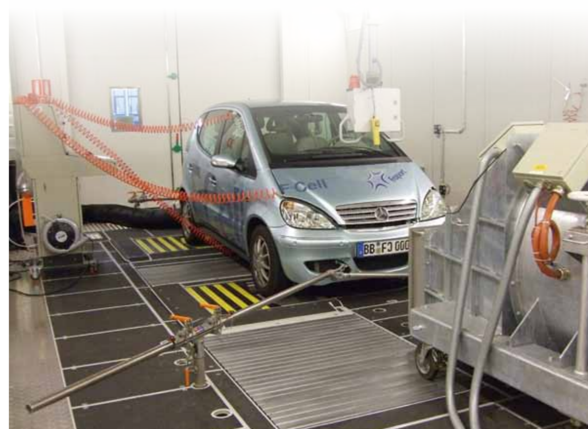
A fuel cell vehicle undergoing testing at the JRC's Vehicle Emissions Laboratory
