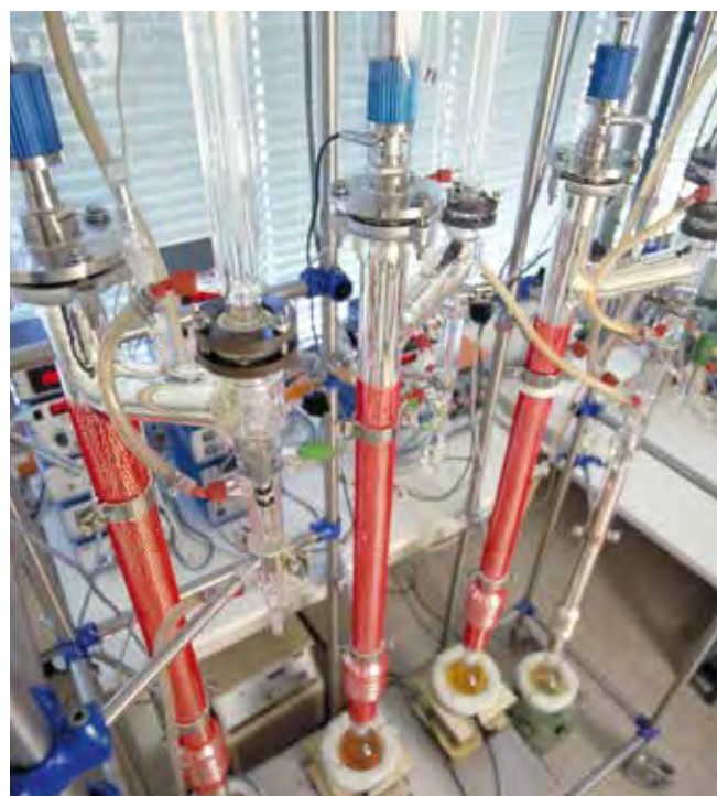
JRC's automated distillation units for wine analysis.
