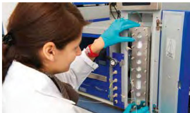
JRC scientists applying field-flow fractionation for characterisation of nanoparticles in feed additives.
