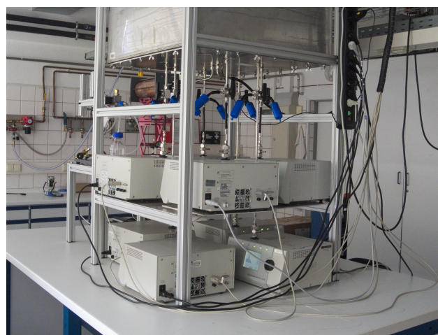
Figure 1. Photo of the measuring setup for the intercomparison of eight units APS 3321.
