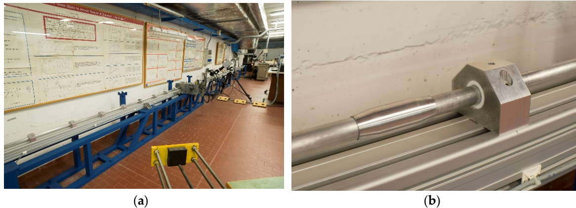
Figure 2. (a) MHPB-SM at the ELSA of JRC; (b) detail of bar-joint and support.
