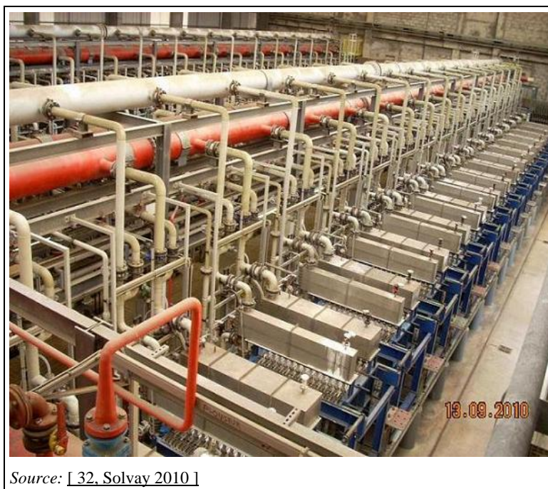
Figure 2.11: View of a membrane cell room equipped with monopolar electrolysers
