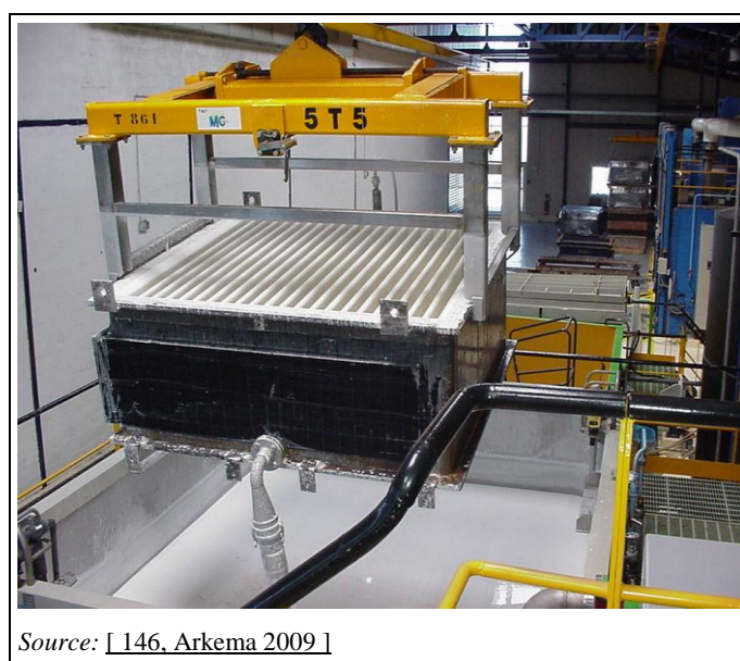
Figure 4.2: View of the deposition of an asbestos-free diaphragm on a cathode
