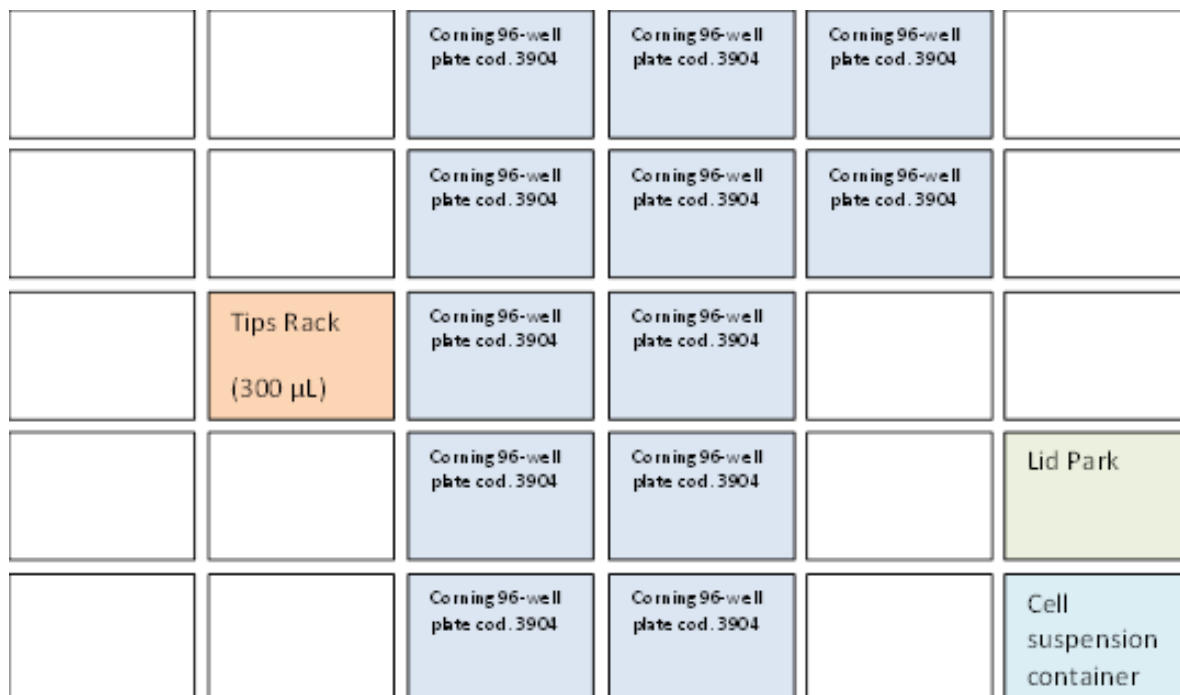
Figure 3: Deck layout for Cell Seeding on Hamilton Starlet Platform on PTP
