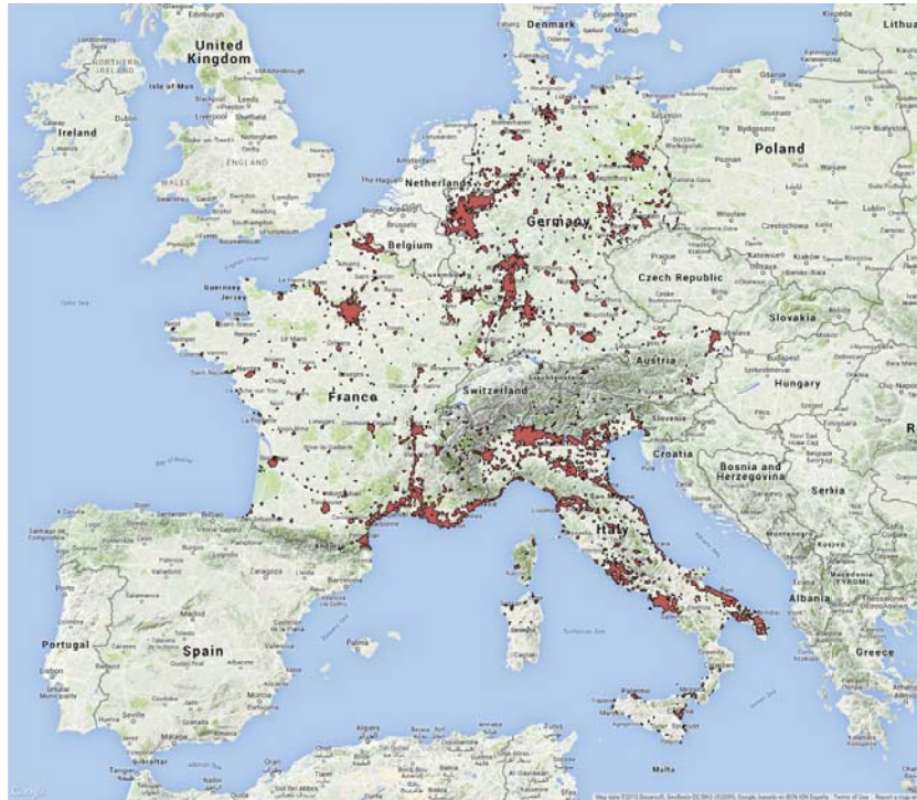
Figure B.3: Densely populated areas used for the analysis of Location Area sizes in urban and rural areas (data taken from [1]).
