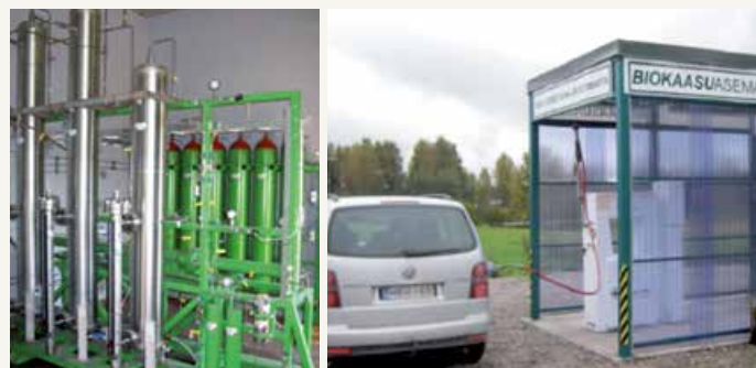
Figure C2 Patented Metener biogas upgrading technology (J. Läntelä) (left) and Kalmari Farm's new fully commercial biogas filling station (O. Pakarinen) (right)
