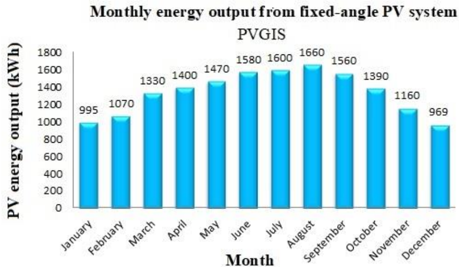
Figure 3: Monthly average power generated by the PV system in kWh
