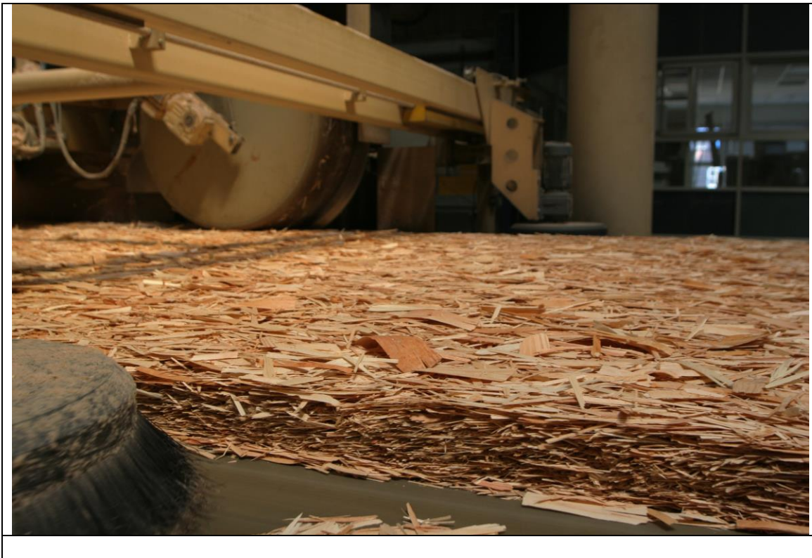
Figure 2.8: OSB mat after forming and trimming
