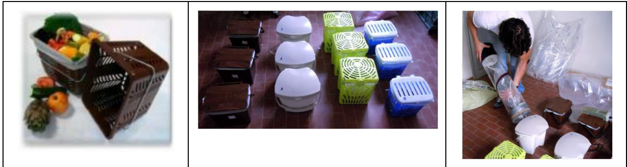
Figure 25: Vented caddy for food waste collection, with compostable bags. Odour test with dynamic olfactometry comparing closed and vented caddies 29
