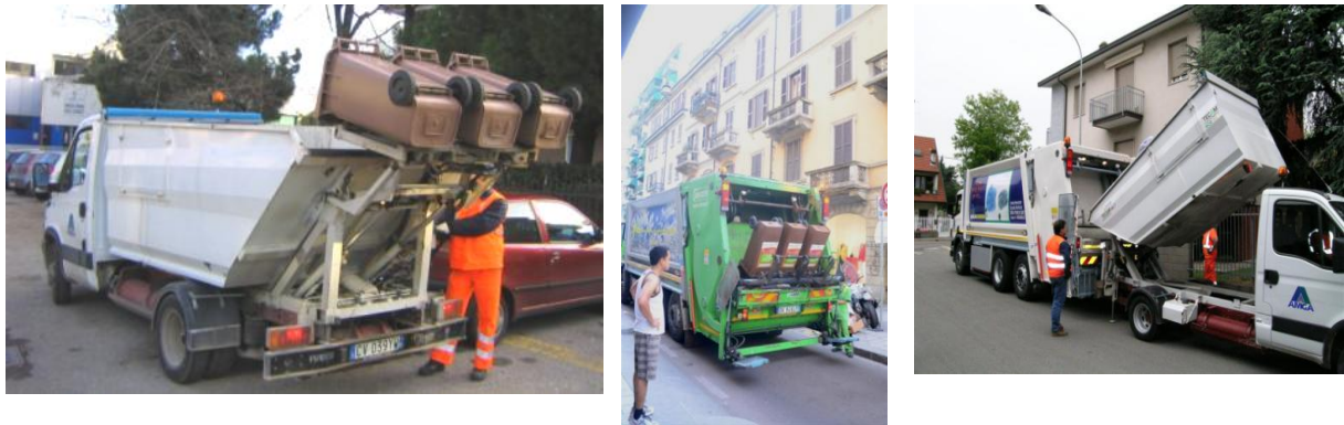
Figure 32: On the most effective and cost saving scheme for food waste collection involves the use of light satellites, a large truck and a limited number of coupling on the street for emptying the satellites.
