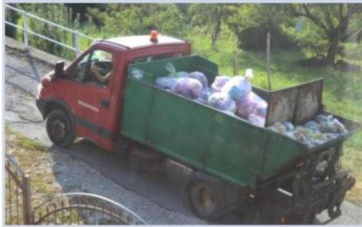
Figure 29: Two-compartment light vehicle for the combined collection of food waste and residual waste to optimize routes and costs
