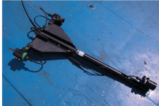
Figure 7. MicroPro free-fall with E_d and L_u sensors located on the lateral side of the fins and an E_u sensor located on the lowest side of the system hub.
