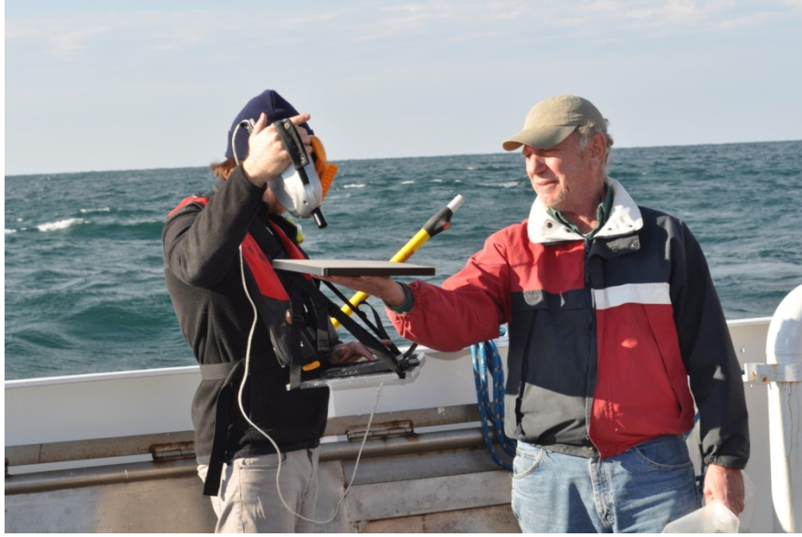
Figure 20. Ryan Vandermeulen and Robert Arnone (USM) aboard the NOAA Ship Nancy Foster , taking above-water radiometric measurements of a gray plaque using an Analytical Spectral Device (ASD) HandHeld Spectroradiometer. The gray plaque has a known BRDF and is used to normalize the un-calibrated radiance measurements to E_S .
