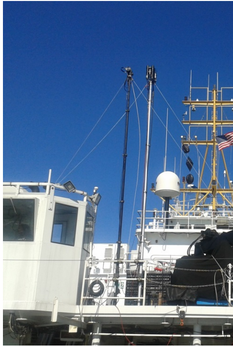
Figure 8. Poles utilized to deploy the various above-water E_d reference sensors. The shadow-band was operated in conjunction with the MicroPro above-water E_d reference sensor to determine the diffuse to direct irradiance ratio required to compute self-shading correction factors for in-water L_u and E_u data.
