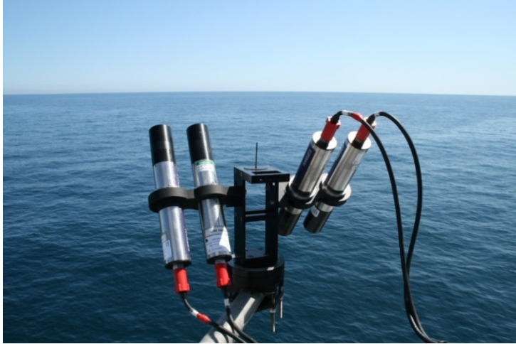
Figure 10. TRIoS radiometer system operated on its mounting frame. One unit (i.e., one L_T and one L_i sensors) has factory-standard 7^\circ FOV. The other unit has custom 3^\circ FOV. The related above-water E_d sensors have been operated in conjunction with all other above-water E_d radiometers.
