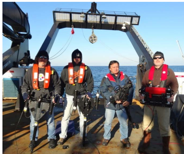
Figure 5. Photograph of the 4 profiling radiometers that were deployed simultaneously off the stern at each station.
