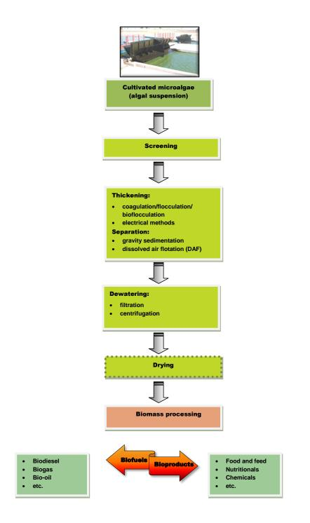
**Figure 2.11.** Process flows diagram of harvesting methods for recovery and dewatering of microalgal biomass. Drying is optional, depending on the selected downstream process for conversion of microalgae to biofuels and/or bioproducts.
