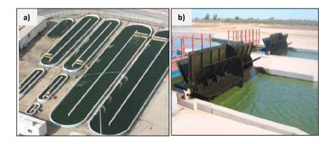
**Figure 2.9.** Examples of ORP systems used for production of microalgae. Inset a) refers to the commercial production of *Nannochloropsis sp.* in Israel [49]; inset b) refers to ORP systems located in California [14].
