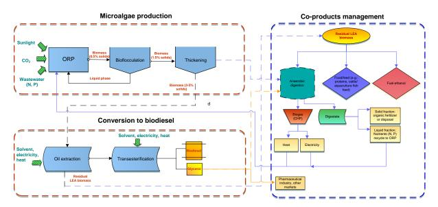
**Figure 4.2.** Main materials and energy inputs and outputs of biodiesel production from microalgae grown in ORP in combination with alternative options for the management of co-products, i.e. LEA biomass, glycerol and solid/liquid fractions of digestate.
