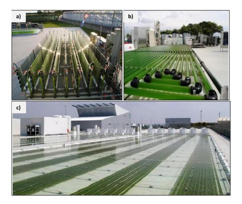
**Figure 2.10.** Examples of demonstration PBRs; the insets a) and b) show tubular PBR in vertical and horizontal configurations, respectively, as developed at Wageningen University (The Netherlands), from AlgaeParc website (<u>http://www.wageningenur.nl/en/Expertise-Services/Facilities/AlgaePARC.htm</u>). Inset c) shows tubular PBRs developed at Fitoplancton Marino SA (Spain), from "Miracless-specialties from algae" website (<u>http://miraclesproject.eu/</u>).
