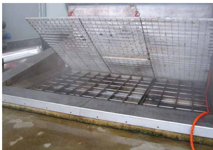
Figure 4: Reception point for liquid co-substrates with different sized grids
