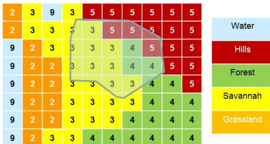
FIGURE 19. EXAMPLE OF AN ACCESSIBILITY MAP FOR A PROTECTED AREA (GREY POLYGON) WHERE LAND COVER CLASSES ARE USED TO DERIVE WEIGHTS AND GENERATE A COST-DISTANCE FUNCTION. HIGH VALUES ARE CORRESPONDING TO OBSTACLES WHILE EASIER ACCESS IS CORRESPONDING TO LOW VALUES.
