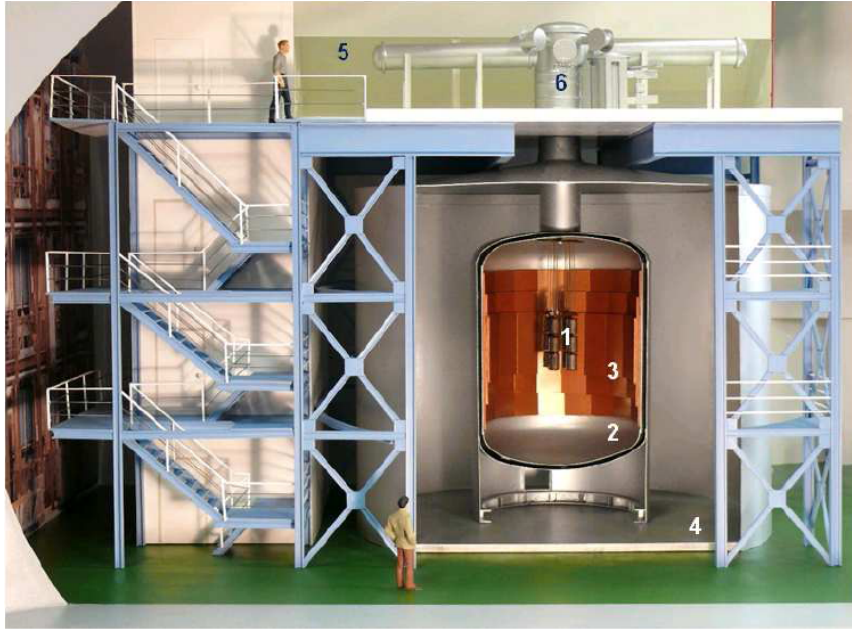
Figure 1: Artist view of the GERDA experiment. The following components are labeled in the picture: (1) the Ge array strings (not to scale), (2) the LAr cryostat, (3) the internal copper shield, (4) the instrumented Water Tank and (5) the Clean Room with the Lock insertion system (6). From [6].
