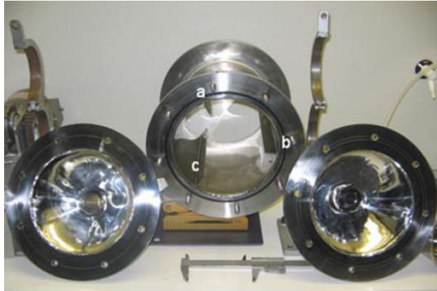
Figure 70. Photograph showing the high-gloss polished inside of the dustiness drum. Also note the three lifter vanes marked a, b, and c at each 120° in the drum.
