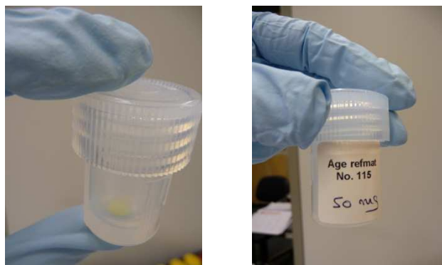
Figure 3: Pictures of the IRMM-1000b units as dried uranyl nitrate in PFA vials
