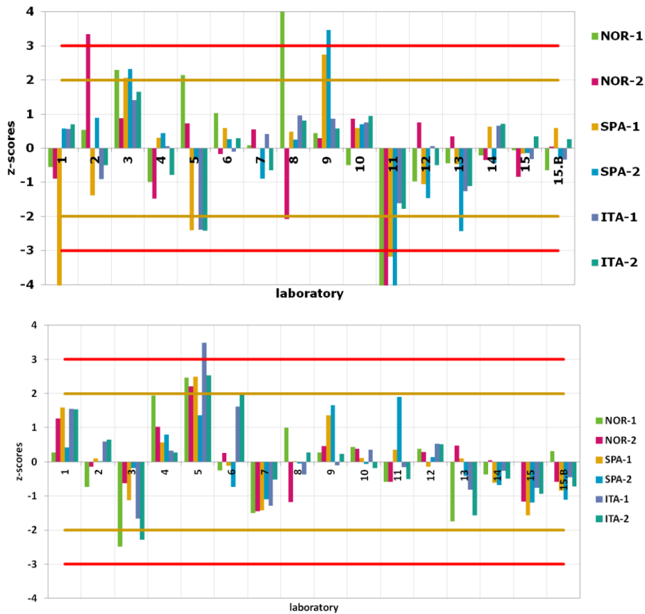
Fig. 18. JRC-IES instruments' (15 and 15.B) performance for the determination of (top) total carbon (TC) and (bottom) elemental carbon (EC/TC ratio) during the ACTRIS inter-laboratory comparison 2013.
