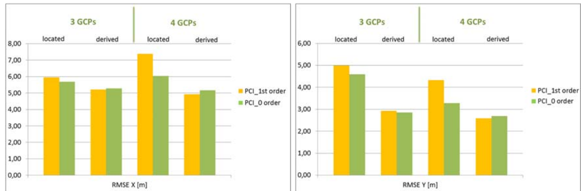
Figure 7: Graph representation of RMSEs comparison between 0 and 1 st polynomial order refinement of MSP images
