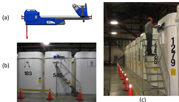
Figure XX: (a) The LMCV device; (b) Device applied in a cask, and (c) Inspector performing weld verification.
