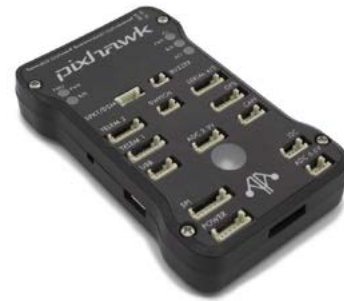
Figure 3. Pixhawk Flight Controller.
