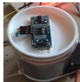
Figure 1. HC-SR04 ultrasonic sensor
