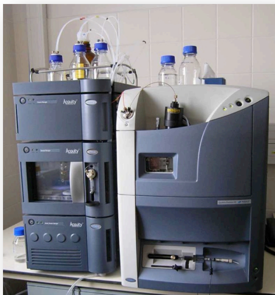
Figure 4 -Liquid chromatograph with triple quadrupole MS/MS (Waters Acquity UPLC with Quattro Premier XE).
