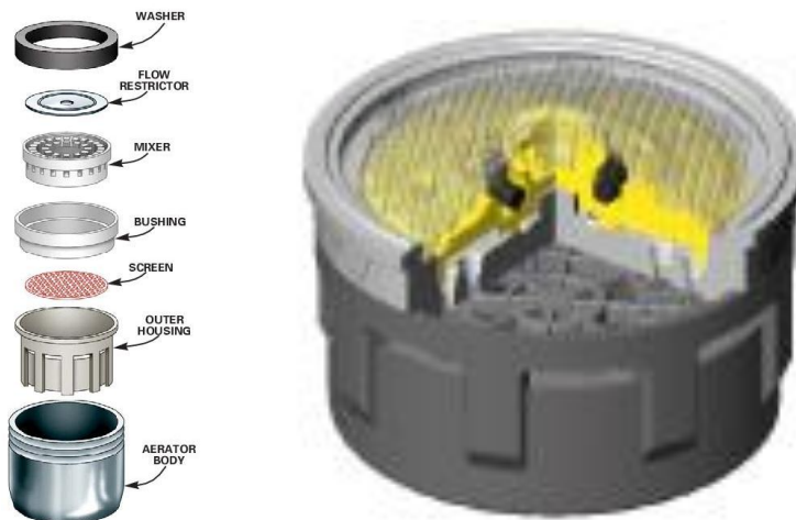
Figure 4.4 Example of a restricted aerator for taps (on the left) 227 and of an aerator with an integrated flow regulator (on the right) 228
