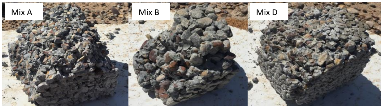
Figure 5. Modes of failure of A, B and D mixes.
