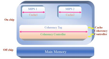
Figure 7. Block diagram for the cache coherency controller
