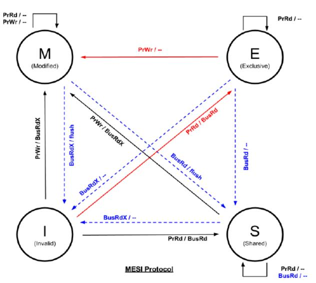
Figure 5. State transition diagram for the MESI protocol
