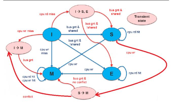
Figure 6. Simple MESI state diagram with state transfer
