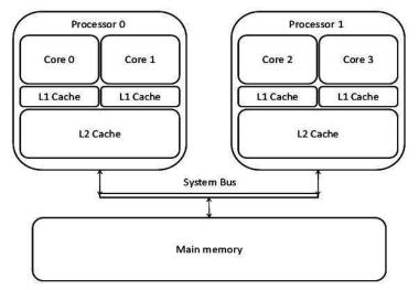
Figure 1. Dual multicore processor.
