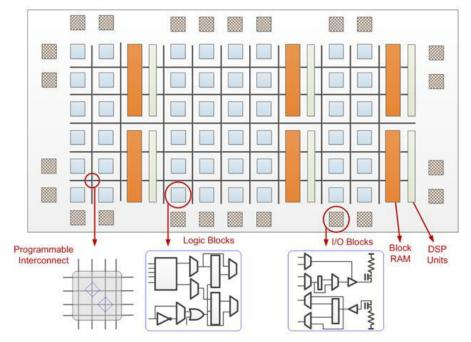
Figure 2. Internal component of FPGA
