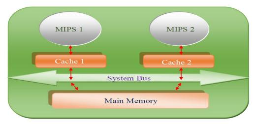
Figure 3. Architecture of dual microprocessor
