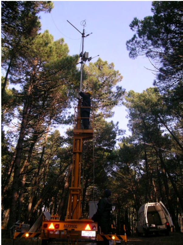
Fig. 60: left: Trailer mast old pinus pinaster site that holds the sonic anemometer and Infra Red Gas Analyser (IRGA) used for flux measurements (in retracted configuration for service). Right: newly erected tower at the pinus pinea site that will hold the measurement equipment.
