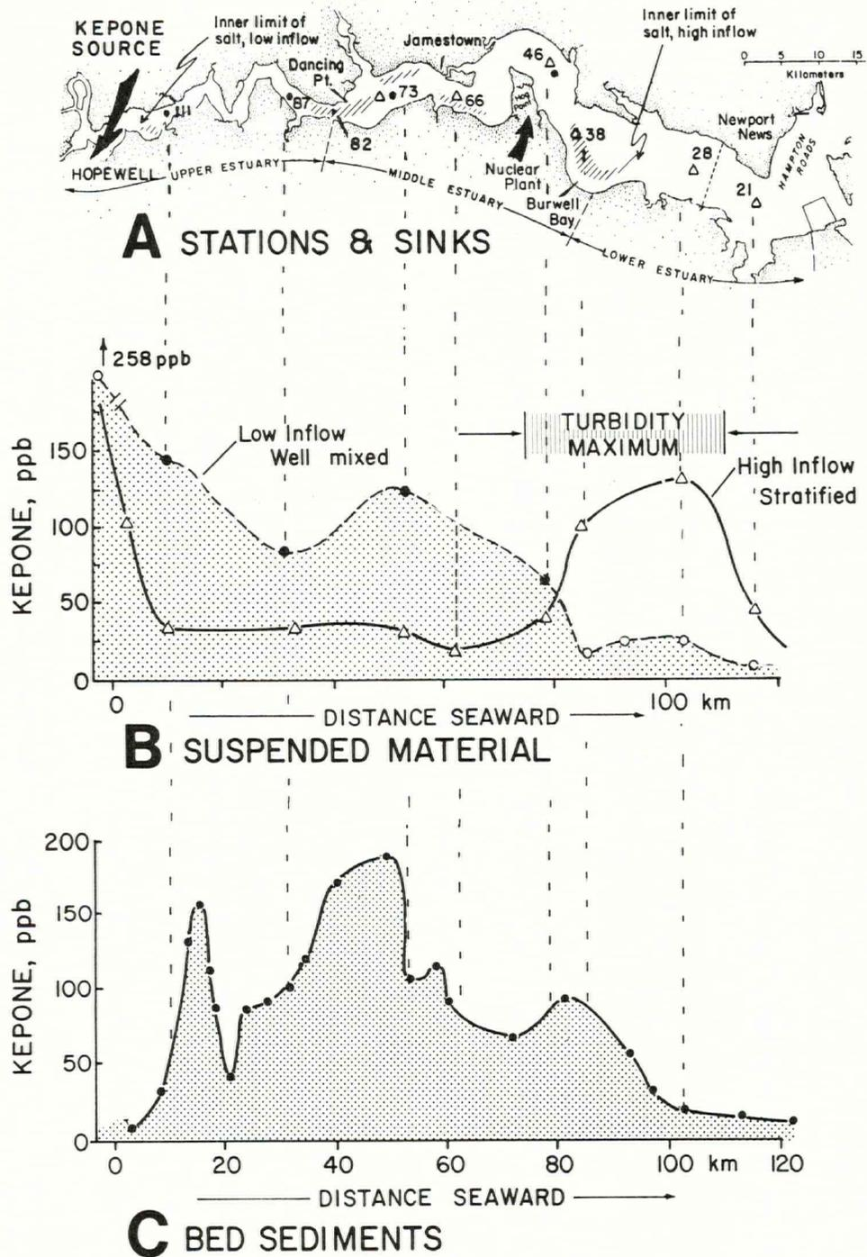
Figure 70. A. Location of anchor stations or suspended sediment and current measurements; hatched, location of major Kepone sinks. B. Longitudinal distribution of Kepone content in total suspended material, average of surface and near-bottom concentrations at low river inflow, August 1977; and high river inflow, April-May 1979. C. Longitudinal distribution of Kepone content in bed sediments from the channel, July 1977.
