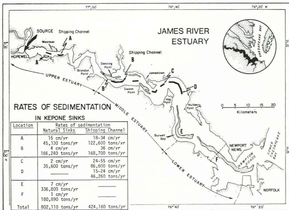
Figure 68. Location of the James River estuary in the southern Chesapeake Bay region, upper right. Zones of deposition, major Kepone sinks, and natural channel, hachured; shipping channel, solid. Rates from radionuclide analyses and from maintenance dredging surveys of the Corps of Engineers, 1965 to 1977.
