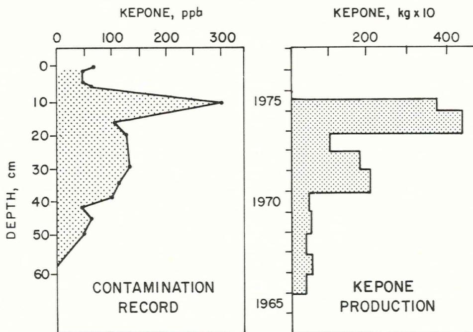
Figure 72. Vertical profile of a nearly complete contamination record, core 82 (Fig. 70A), in relation to Kepone production from sales records, 1966 to 1975.
