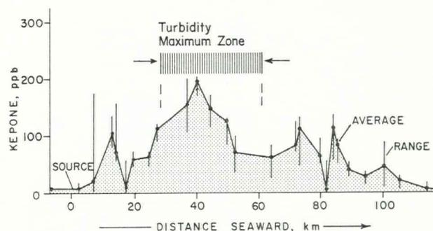
Figure 69. Distribution of Kepone concentrations in bed sediments with distance seaward along the estuary. Based on an average of three sample sets collected from channel stations (> 4 m depth) between December 1976 and July 1977.
