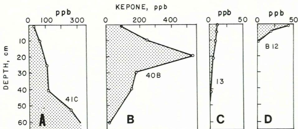
Figure 71. Vertical profiles of Kepone content in cores from different sedimentation zones. A, relatively fast sedimentation in shipping channel; B, intermediate sedimentation, natural channel; C, lower estuary; D, slow sedimentation, middle estuary shoal.
