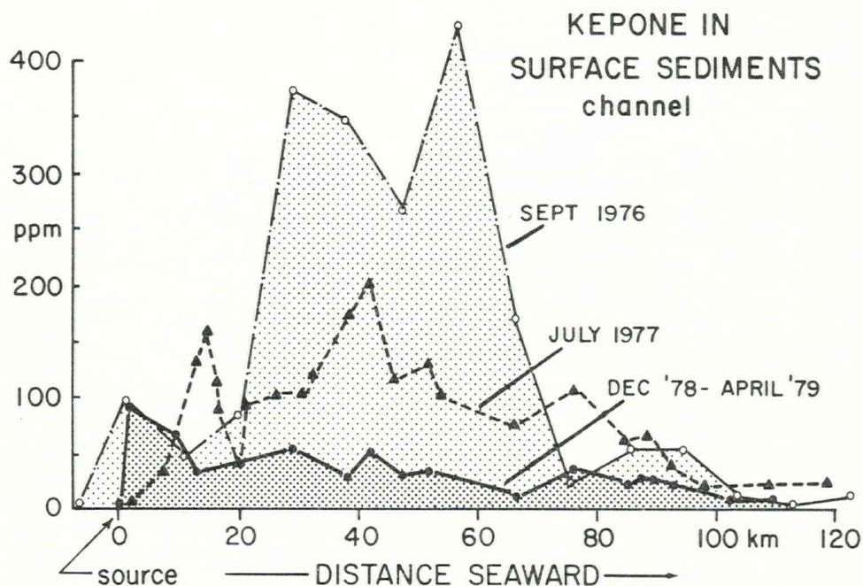
Figure 73. Longitudinal distribution of Kepone in surface sediments at different times, September 1976, July 1977, December 1978 to April 1979. Decreasing concentrations indicate gradual "recovery" in the middle estuary.
