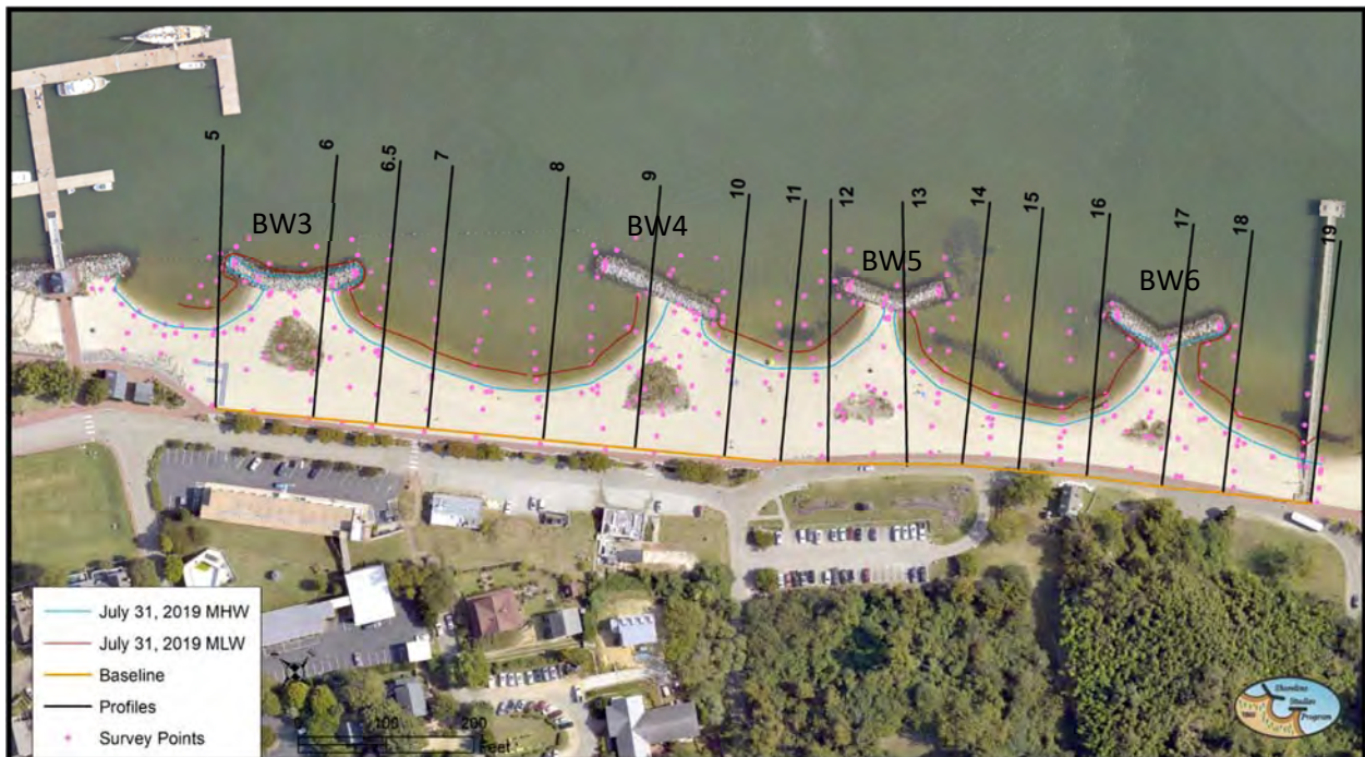
Figure 3-2. Data points collected at Yorktown to determine elevation changes at the site since installation. Also shown are the measured mean high water and mean low water lines and the cross-sectional profiles exported for the project.
