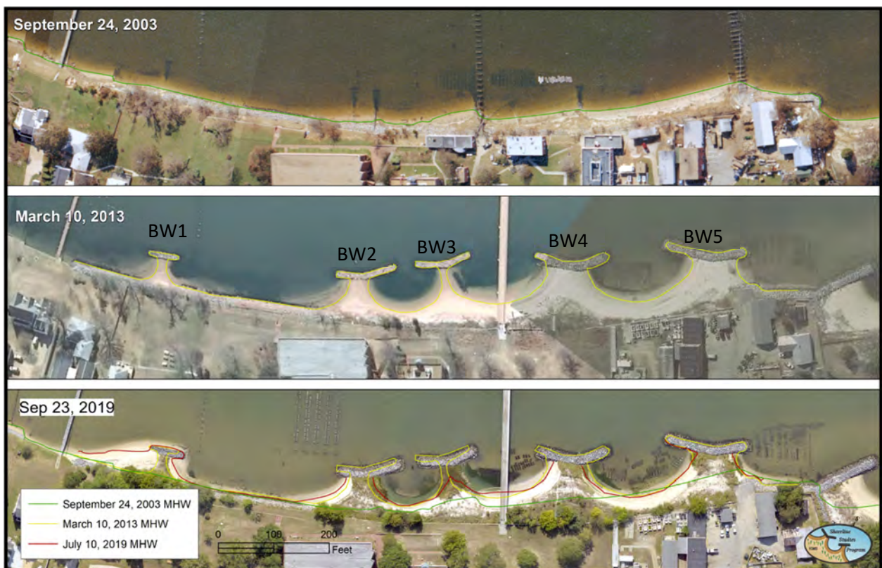
Figure 4-1-10. Shoreline change between 2003 and 2019 at the VIMS breakwaters. The 2003 pre-installation date is shown for reference. The 2003 and 2013 shorelines are approximately mean high water based on the digitizer's best guess of the features shown. The 2019 shoreline is from the survey data.
