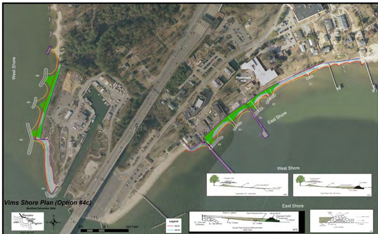
Figure 4-1-8. Shore protection plan designed for VIMS after Hurricane Isabel significantly impacted its shoreline.
