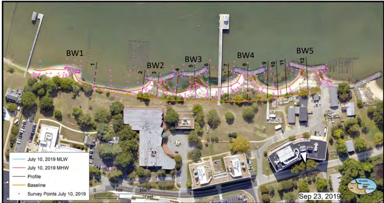
Figure 3-1. Data points collected at VIMS to determine elevation changes at the site since installation. Also shown are the measured mean high water and mean low water lines and the cross-sectional profiles exported for the project.
