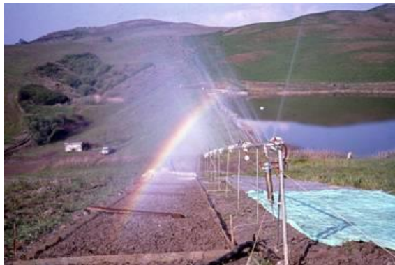
Figure 3 – Rain simulator to define soil erodibility.
