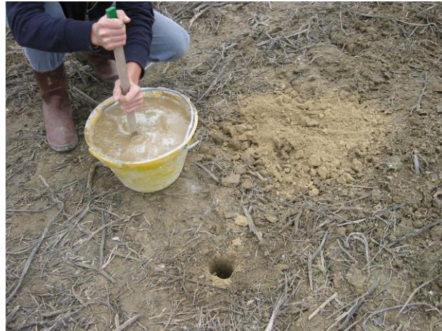
Figure 6 -Preparatory phase of the plot of land for the installation of the hollow housing plates to measure moisture content for each soil horizon
