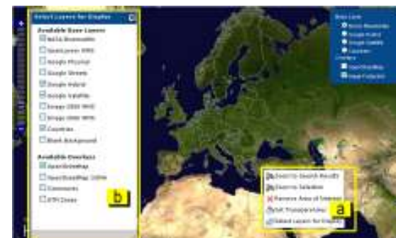
Figure 6: User interface. Right mouse click context menu [a] and select layers to be available in the layer selector [b]
