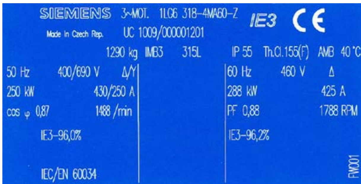
Figure 10 Rating plate according to IEC 60034-1 for 3-phase 4-pole IE3 motor: at 50 Hz with 250 kW and 96.0% efficiency (1488 rpm), \cos \phi 0.87; 400 V, 430 A; at 60 Hz with 288 kW and 96.2% efficiency (1788 rpm). power factor 0.88 460 V, 425 A; (Source: Siemens online catalogue 2013)
