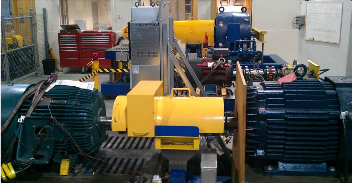
Figure 11 Measurement set-up for measurement of motors with variable frequency drives at the Hydro Quebec motor testing laboratory, near Montreal, motor under test is to the right, the torque and speed meter in the middle (under yellow cover), the load machine is to the left, the VFD is placed outside the picture (Source: Pierre Angers 2013)
