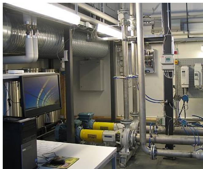
Fig 6 Laboratory test setup comprises a water tank, various piping, a centrifugal pump, an induction motor, and a frequency converter.
