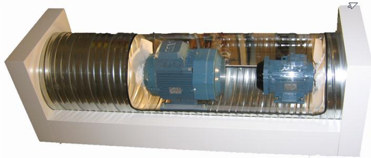
Figure 3, 11kW 3000rpm motors. IE2 induction motor frame size 160 (left), High output SynRM frame size 132 (right).
