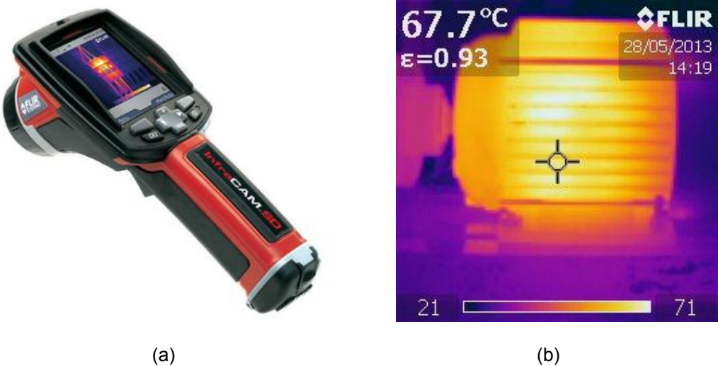
Figure 7 – Infrared camera (a) and thermal image (b).
