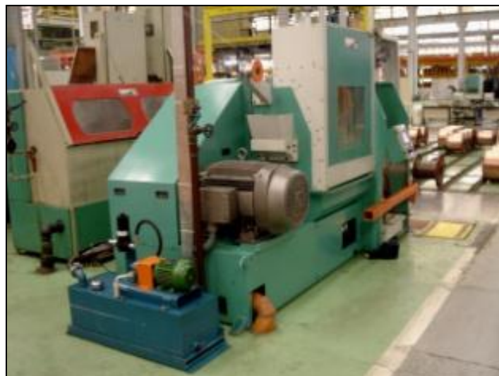
Figure 8. Wire drawing machine with PM motor
