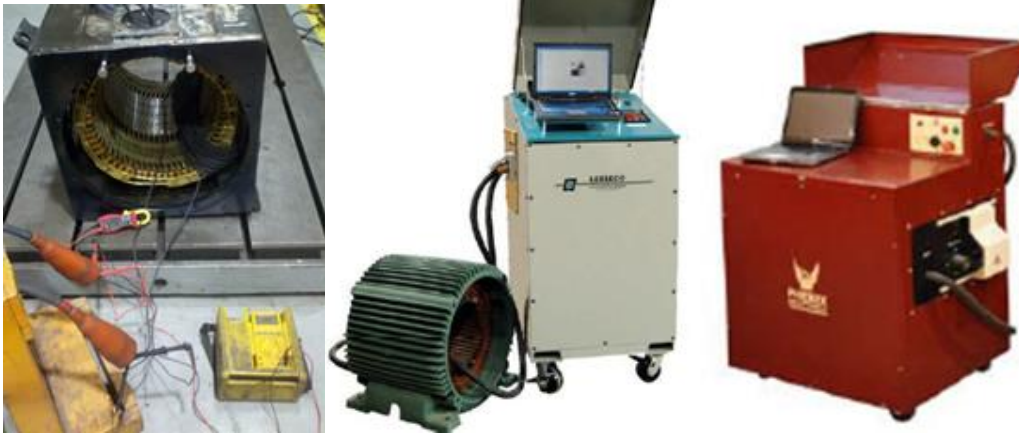
Figure 4: Picture of the EASA Loop Test and commercial core loss testers.
