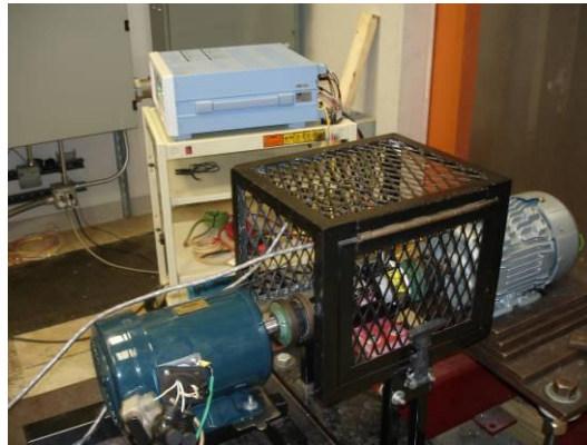
Fig 1: A 1hp motor setup to investigate unbalance effects
