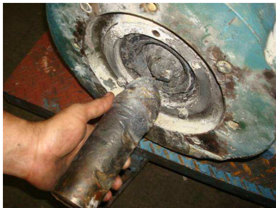
a) Front bearing of a damaged machine.
