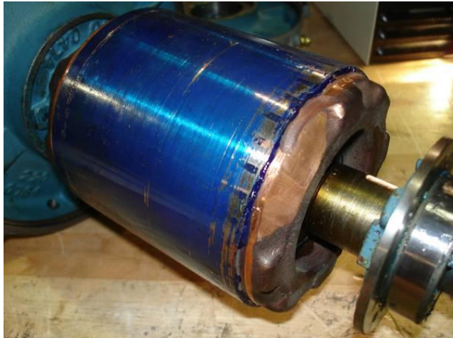
Fig. 18: Die-cast copper rotor for induction motor
