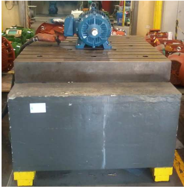
a) Rigid base according to IEC 60034-14.
