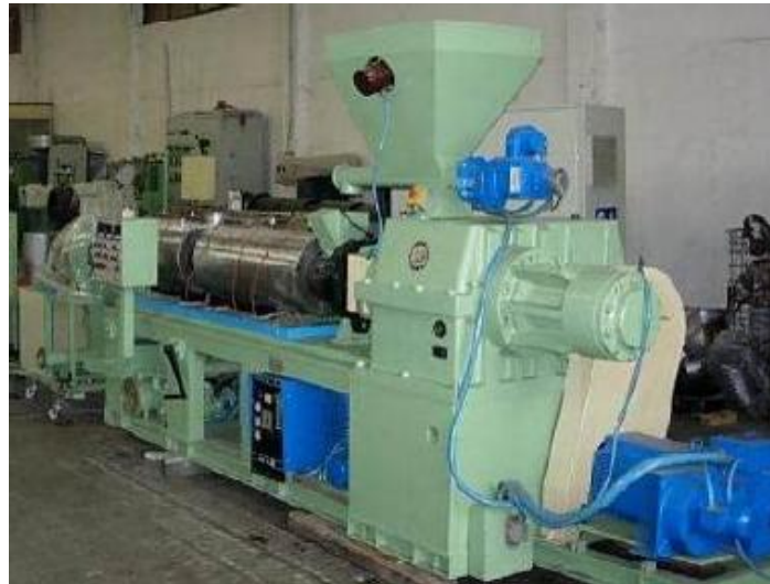
Figure 11. Extrusion machine with PM motor
