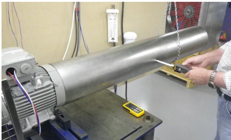
Photograph 1: measuring the air velocity in the duct: TEFC motor
