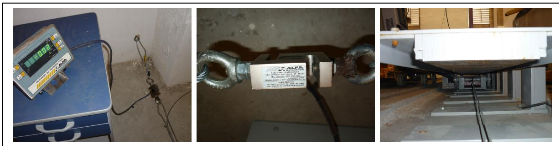
Figure 3 – Traction Force measurement
