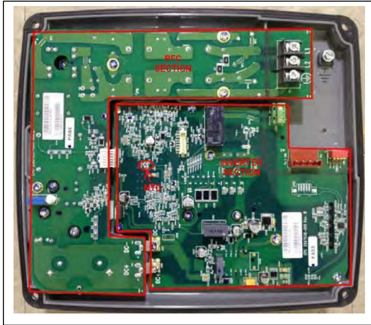
Figure 1 Controller sections and location of thermistor
