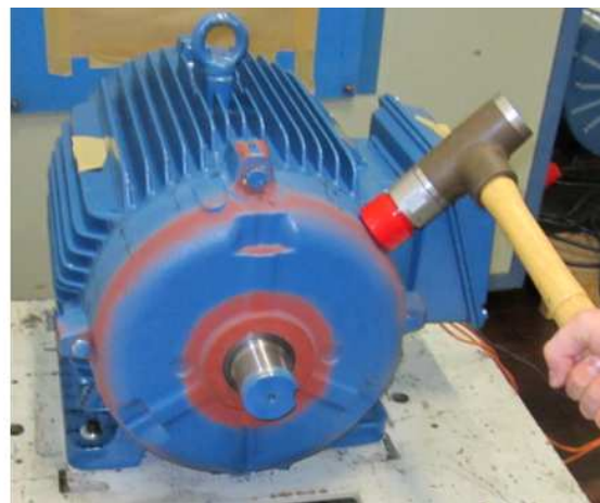
Figure 2: Acquisition points of the response and excitation signals for the modal analyses.
